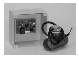
The *ISIMET* Emergency Shower Monitoring Unit is a companion component to the ISIMET Utility Controller System. The unit is provided with a micro-flow switch, time delay circuit, junction box, and mounting hardware. The unit is not provided with a power source and must derive 24-vac operating power from the companioned Utility Controller.
